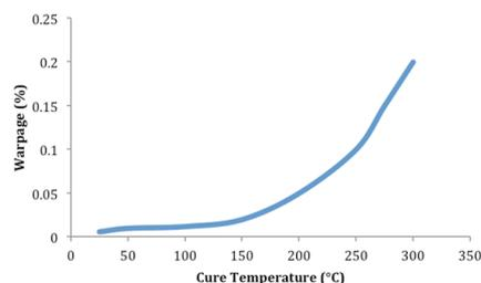
Figure 1: Degree of warpage vs. curing temperature.
