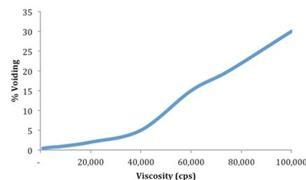
Figure 2: Percentage voiding vs. material viscosity.
