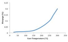
Figure 1: Degree of warpage vs. curing temperature.
