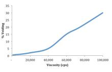
Figure 2: Percentage voiding vs. material viscosity.
